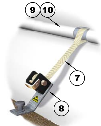
TYPICAL End Wall Tubing to Anchor Winch Connection
